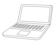
Power rating = 75 Watts Running cost: 2p (per hour)
